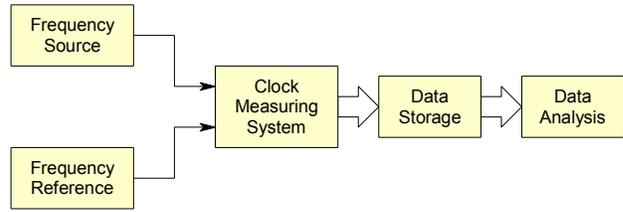
Figure 2. Basic Clock Measuring Setup
