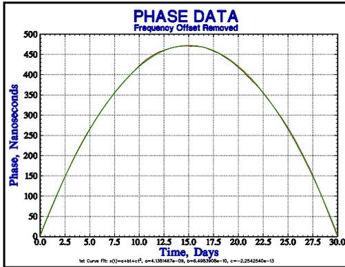
Quadratic shape is due to freq drift - can now begin to see phase fluctuations.
