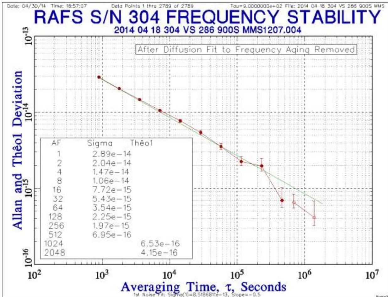
Figure 3. ThêoH Stability Plot for a GPS Rubidium Clock
