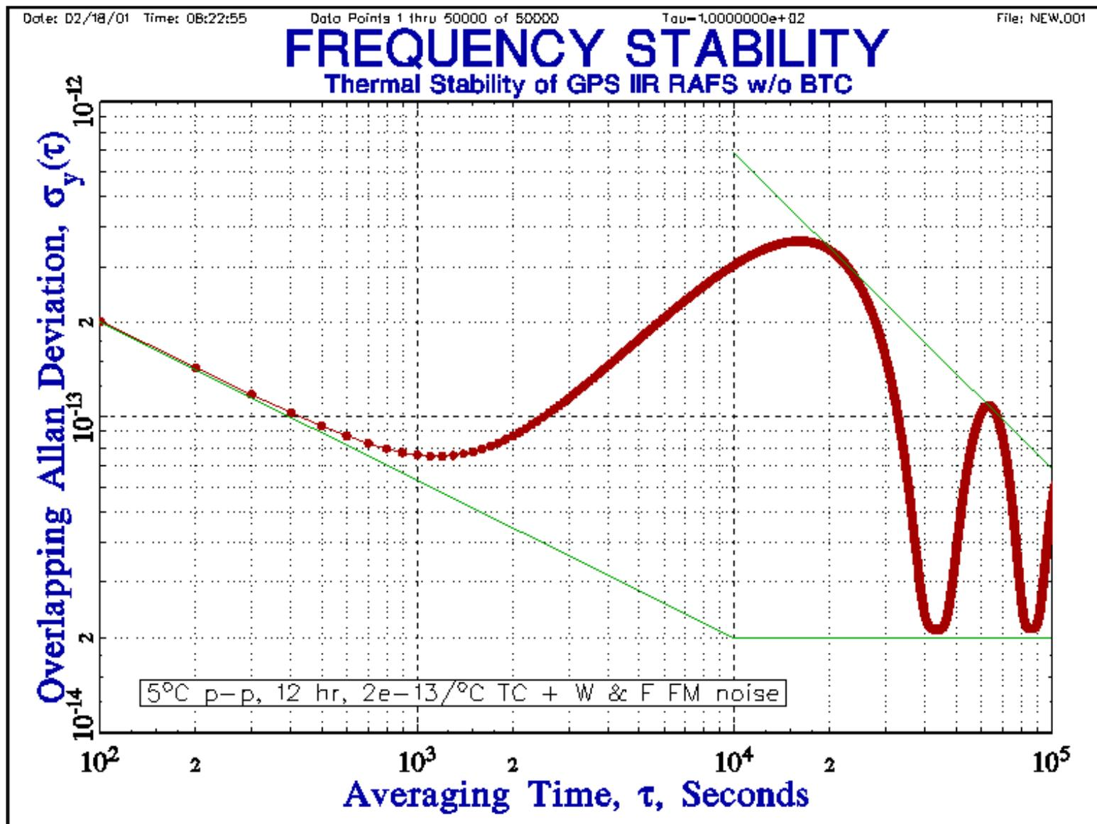
The same general expression applies to the effect of vibrational modulation on the stability of a frequency source. It should be noted that the envelope of the resulting stability plot shows both (at the top) the vibrational FM ( $1 \times 10^{-9} \cdot \sqrt{2}$  rms at  $1/2 \cdot f_{\text{vib}}$ ) and the noise ( $1 \times 10^{-12} \tau^{-1}$ ). Minima occur at averaging times equal to multiples of the vibration period.
