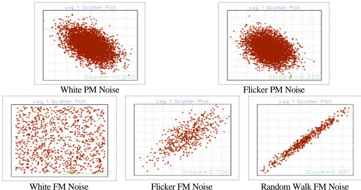
Figure 2. Lag 1 Scatter Plots for Frequency Data
