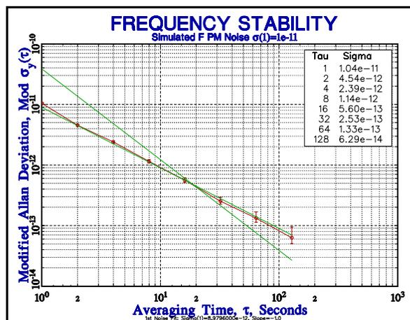
The W and F FM noise slopes are both  $\approx -1.0$  on the ADEV plots, but they can be distinguished as  $-1.5$  and  $-1.0$  respectively on the MDEV plots.
