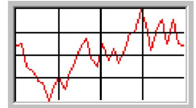
Frequency data is often plotted the same way, simply because that is the way plotting is usually done. But a better presentation is a flat horizontal line between the frequency data points. This shows the averaging time associated with the frequency measurement, and mimics the analog chart record from a counter.
