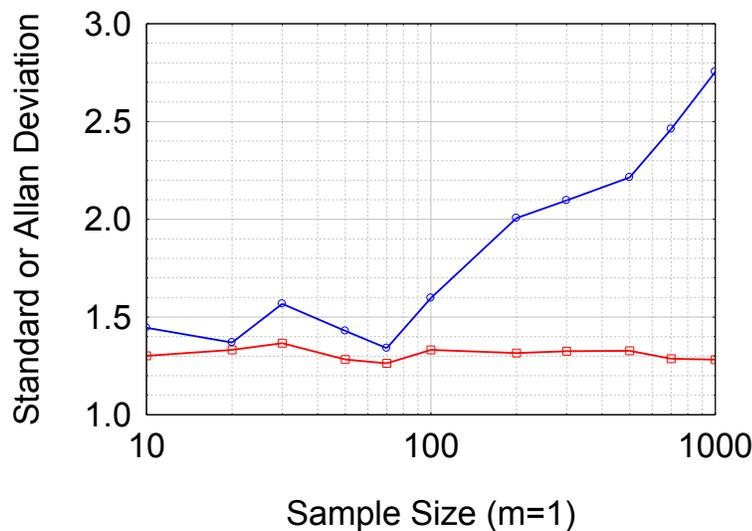
Figure 1. Convergence of Standard and Allan Deviation of Flicker FM Noise. The standard deviation depends on the sample size for flicker FM noise, while the Allan deviation does not and is therefore a better measure of frequency stability.
